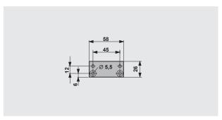
**Upstand hinge bracket**For fixing the arm to particularly narrow door frames.
