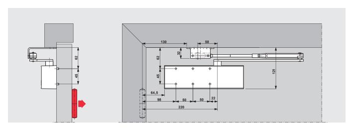
(Example refers to left-hand (IS06) door; mirror image applies to right-hand (IS05) door). With this fixing method, the closing force is approximately 20Nm (for doors up to 950mm)
